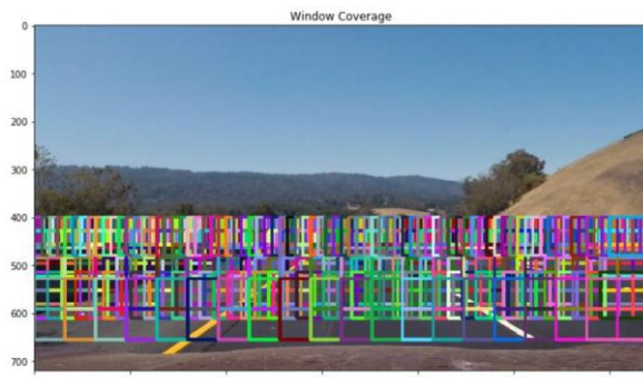
Fig. 3. The regional proposal network running on only lower half of the image, avoiding to run the region with least probability of object density
