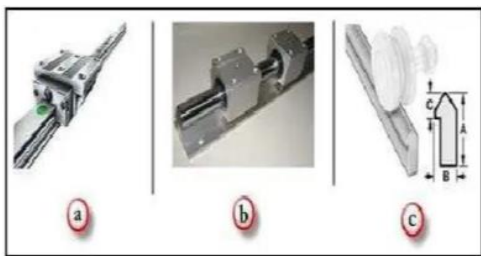
(a) Rail & guide (b) rod & bushing (c) v-groove Fig. 4. Types of linear motion systems
