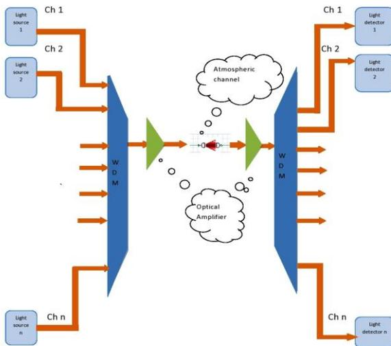
Fig. 1. Proposed WDM-Ro-FSO communication system
