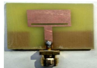
Fig. 8. Fabricated front rectangular patch antenna
