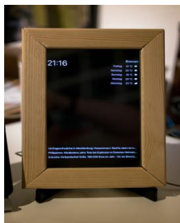
Fig. 1. Smart mirror with LCD display at the backend
