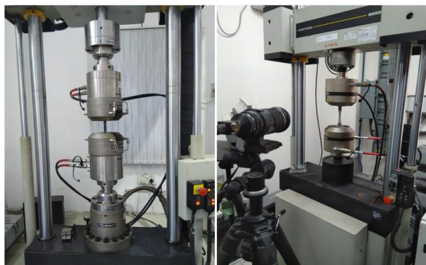
Fig. 5. Experimental setup for: a) Fatigue, b) DIC
