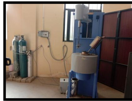
Fig. 1. Bottom stir casting
