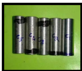
Fig. 4. Wear test specimen
