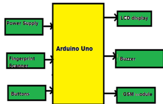
Fig. 1. Block diagram of biometric voting machine
