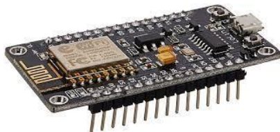
Fig. 1. NodeMcu for Wi-Fi and connectivity
