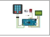
As shown in below block diagram power supply given to controller Arduino Mega 2560. 4X4 matrix keypad is use as input to controller. Depending input controller will give PWM signal to motor driver L298N, which drives dc motor in such
