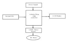
As shown in below block diagram power supply given to controller Arduino Mega 2560. 4X4 matrix keypad is use as input to controller. Depending input controller will give PWM signal to motor driver L298N, which drives dc motor in such way that we get desired output. The input count and output results will display on LCD display connected to Arduino Mega respectively.
