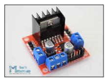
Let's take a closer look at the pin-out of L298N module and explain how it works. The module has two screw terminal blocks for the motor A and B, and another screw terminal block for the Ground pin, the VCC for motor and a 5V pin which can either be an input or output.
