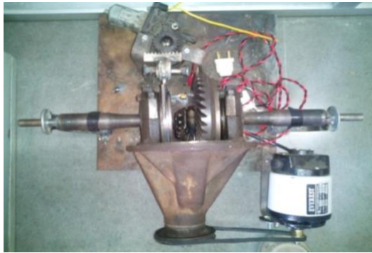
Fig. 3. Fabricated view of differential locking system
