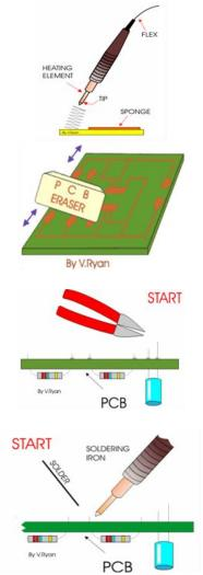
A PCB eraser is used to remove any film from the tracks. This must be done carefully. Because the film will prevent good soldering of the components to the PCB. The tracks can be checked using a magnifying glass. If there are gaps in the tracks, sometimes they can be repaired using wire but usually a new PCB has to be etched.
