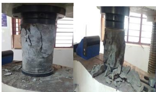
Fig. 4. Cube and cylinder during testing
