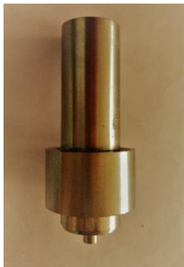
Fig. 3. FSW tool with cylindrical pin
