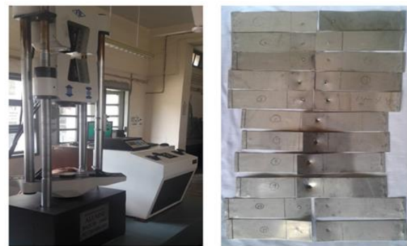
Fig. 5 (a) UTM setup, (b) Specimen after checking tensile strength
