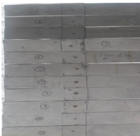
Fig. 3. Overlapped joining of ASS (316L) welded with difference parameter range
