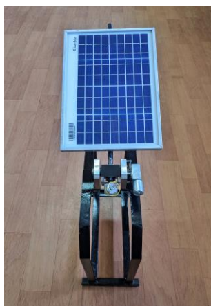
Fig. 2. Hardware implementation of autonomous solar panel
