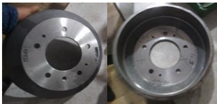
Fig. 2. Casting under case study (Break Rear Drum 180 no.)
