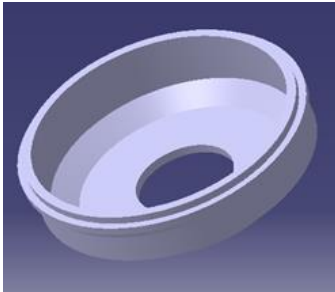
Fig. 3. 3D Model of final casting
