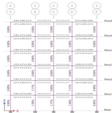
Fig. 2. Elevation Steel in Percentage using Conventional Brick in Dead load
