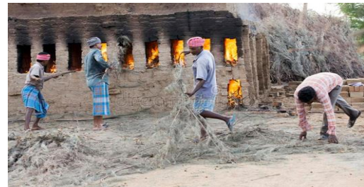
Fig. 1. Burning of red brick
