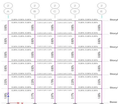
Fig. 3. Elevation Steel in Percentage using Conventional Brick in Dead load
