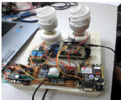
Fig. 6. Full circuit connection with PIR sensor
