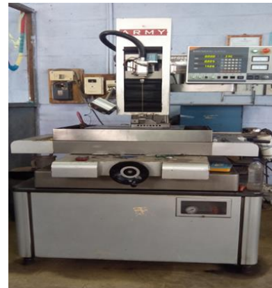
Fig. 1. Photograph of the experimental apparatus of the EDM
