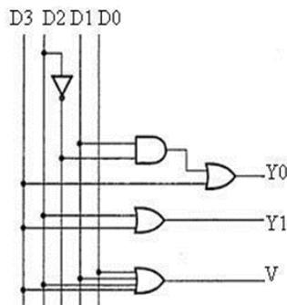
Fig. 1. Existed block diagram of priority encoder
