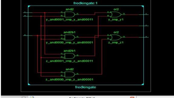
Fig. 5. RTL schematic of URL Gate
