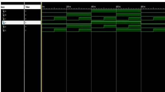
Fig. 6. Simulation of fredkin gate
