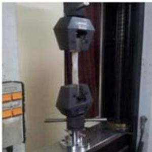
Fig. 3. Specimen during testing
