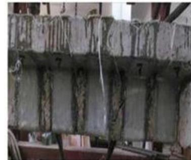
Fig. 8. Crack in web portion
