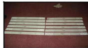
Fig. 1. Specimens for tensile testing of woven glass/epoxy composite
