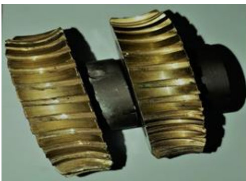
Fig. 2. Two different modes of failure in gear, one is due to wear and other is due to misalignment
