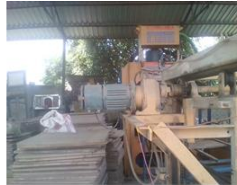
Fig. 3. Stacker assembly of ash brick factory
