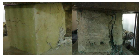
Fig. 2. (a) Control concrete cube failure, (b) Plastic concrete cube failure
