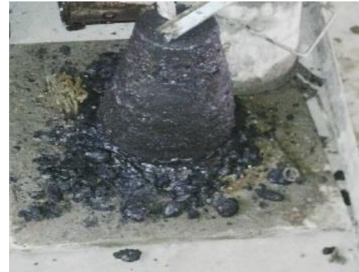
Fig. 4. Determination of Slump value on SDA fresh Concrete
