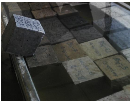
Fig. 7. Preparing SDA concrete cubes for compressive strength test
