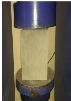
Photo-5: Compression testing machine after placing specimen
