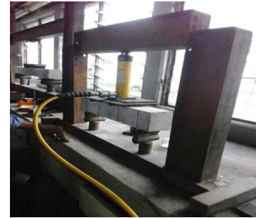
Fig. 8. Laboratory testing of reinforced concrete beam
