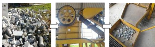
Fig. 4. Process of Crushing and Sieving Recycled Aggregates; (a) Concrete Waste, (b) Crusher Machine, (c) Sieve Method
