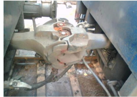
Fig. 2. Illustration of AAR (H) type Tight Lock Center Buffer Coupling of ICF Coaches
