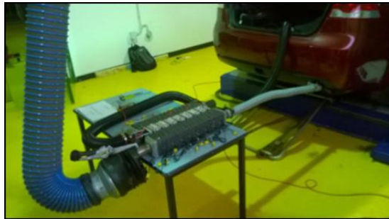
Fig. 5. Lab setup of heat recovery system
