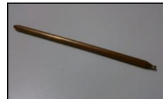
Fig. 2. Cylindrical copper/water heat pipe
