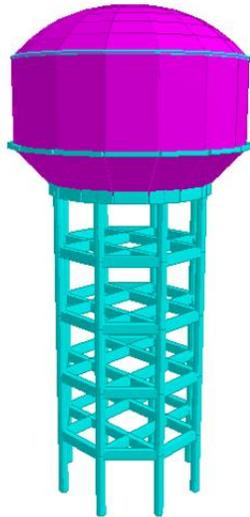
Fig. 6. Finite element model in Stadd.ProV8i
