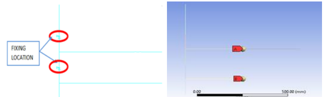
Fig. 8. FE model of Bracket Rack assembly with Boundary condition and mass applied
