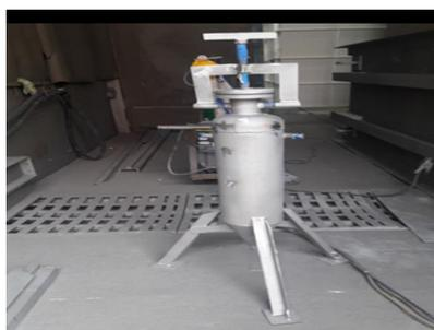
Fig. 3. Portable shot blasting machine
