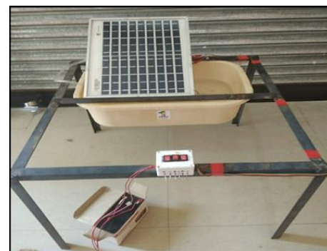
Fig. 2. Experimental set up for combine PV TEG setup
