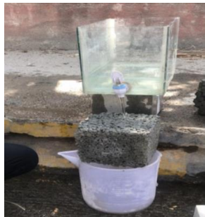
Fig. 4. Collection of water by passing it through concrete block
