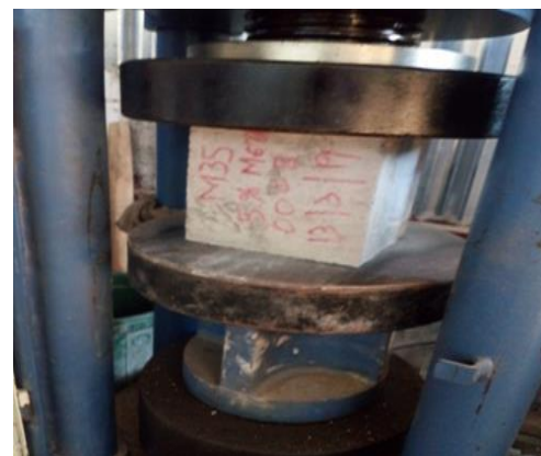
Fig. 1. Compression strength testing machine
