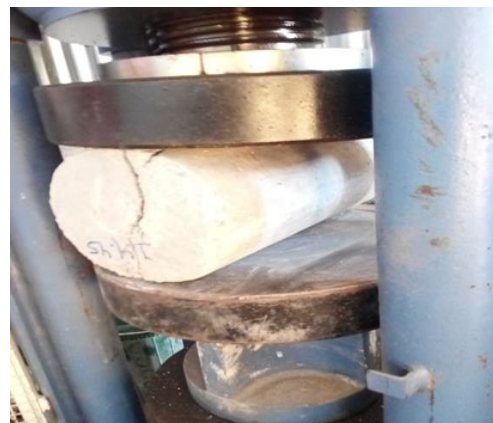
Fig. 2. Split tensile strength test machine
