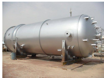
Fig. 1. Horizontal Retention Vessel
