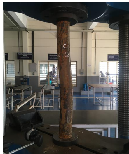
Fig.12. Specimen with 1 % glass fibre After Loading
