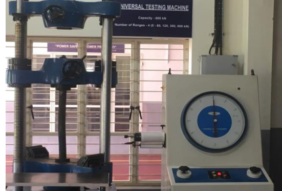
Fig. 6. Test setup for compression test
