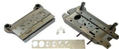
Fig. 1. Progressive Die with Scrap Strip and Stampings
