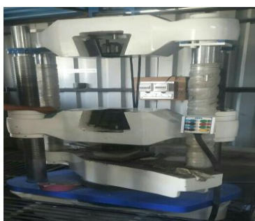
Fig. 1. Compressive strength test
