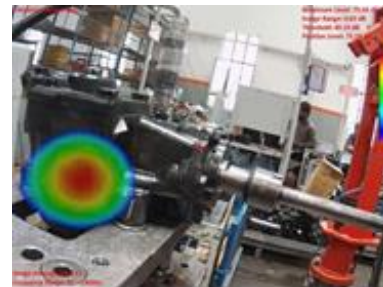
Fig. 4. Localization of noise source
