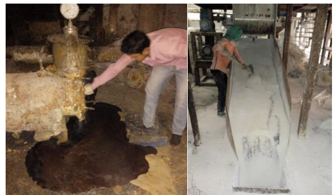
Fig. 2. Removing filter pan and spading powder mixture
