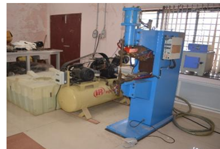
Fig. 1. Resistance spot welding machine
