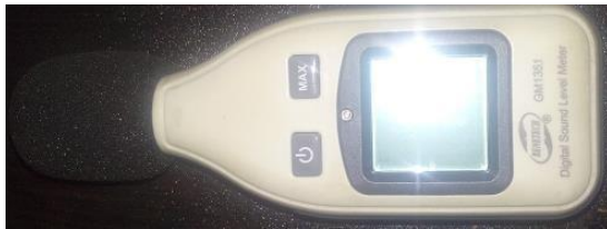
Fig. 4. DB Meter used for noise measurement
