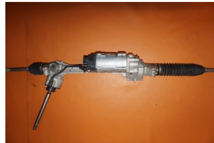
Fig. 4. Rack and Pinion
