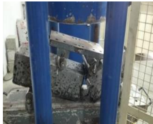
Fig. 1. Flexural beam test of specimen
