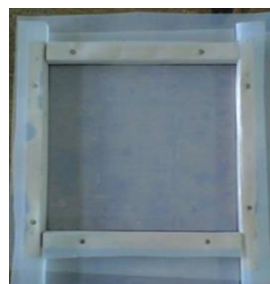
Fig. 3. Mould used for fabrication of the composite
