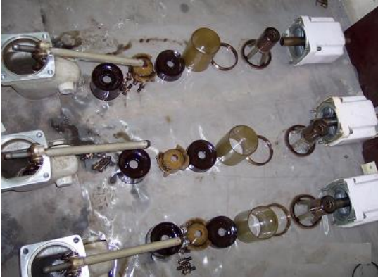
Fig. 3. Internal components of MOCB
