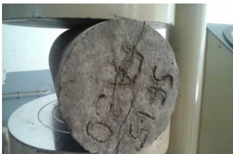
Fig. 2. Split tensile strength test on SFRC specimen
