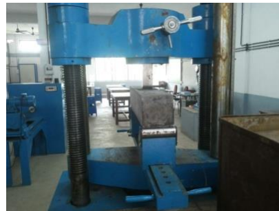
Fig. 3. Flexural strength test on SFRC specimen
