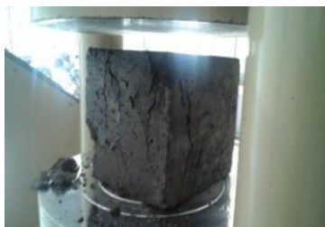
Fig. 1. Compression test on SFRC specimen
