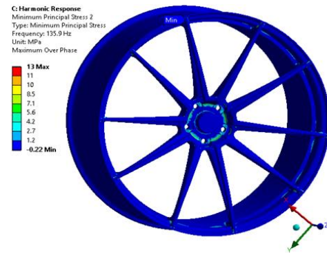
Fig. 12. Min. principal stress of -0.22 MPa is observed
