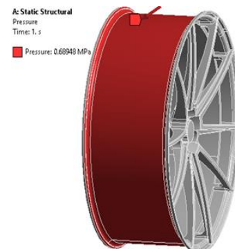
Fig. 2. Loading and boundary conditions
